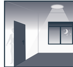
After hold time, the sensor dims the lamp at a low light level if no new motion trigger
